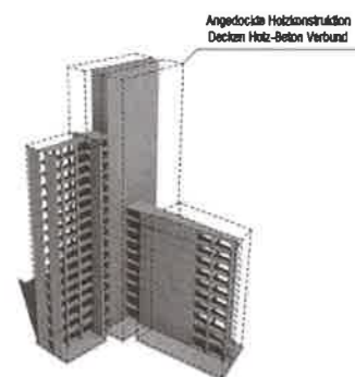
Fig. 1: Basic concept of the bearing structure
